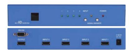
This switcher is a high performance HDMI switcher with IR remote and RS-232 controls. It allows your various HDMI sources to share one HDMI display. Simply pressing one button to select your desired HDMI source for display on the TV/monitor.
