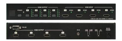
This matrix is the ideal solution for connecting all your HDMI devices, and thanks to the included remote this system gives you complete control over your media environment. Furthermore, the HDMI V1.3 Matrix can transfer Deep Color video and bit stream digital audio with maximum performance.
