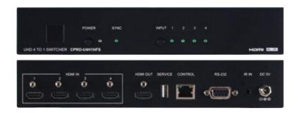
This switcher is the most advanced HDMI solution for Ultra High-Definition (UHD) signal distribution. This unit allows for the switching of any of four 3G HDMI input signals to a single 3G HDMI display. With support for resolutions up to 4K@30Hz, 36-bit Deep Color, HD audio as well as other features defined by the HDMI 1.4 specification. Multiple control interfaces are available including RS-232, Ethernet (WebGUI & Telnet), IR remote, and front-panel buttons making operation easy and intuitive.
