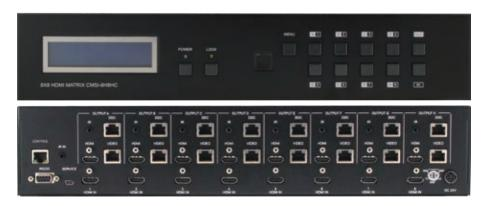
This matrix has simultaneous HDMI and Dual-CAT6 outputs that connect 8 HDMI sources to 16 displays. It features 8 HDMI outputs and each HDMI output is mirrored to provide a Dual-CAT-Cable output which runs simultaneously. Connect a compatible receiver to each of the Dual-CAT-Cable outputs to extend the HDMI signal up to 45 meters (1080p, 8-bit) for multi-room connectivity.
