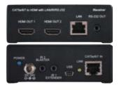
This splitter is designed to receive an HDBaseT signal from a compatible transmitter or matrix unit. It features full HDBaseT convergence allowing the transmission of video, audio, control (IR/ RS-232), 24V PoC (Power over Cable), and LAN serving over a single CAT5e/6/7 cable up to 100m.
