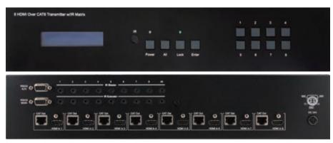
This transmitter supports the transmission of uncompressed video (up to 1080p@60Hz) and multi-channel digital audio from eight HDMI sources to eight HDBaseT outputs over a single CAT5e/6/7 cable (up to 100m) for each output. It supports passing 7.1 channel LPCM digital audio as well as standard Bitstream and HD Bitstream audio formats.
