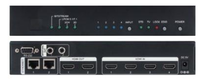
This switcher is a four inputs & two outputs HDMI switcher. The output ports support Audio Return Channel (ARC) from a compatible ARC TV and HDMI Ethernet Channel (HEC) following the HDMI specification. This unit provides an S/PDIF link from the HDMI signal and output through the ARC port to an AVR/amplifier to get audio from the sink.
