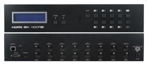
This matrix supports the transmission of video (resolutions up to 4K@30Hz & HDCP 2.2 compliant), multi-channel digital audio, and control via IR, RS-232, Telnet or WebGUI from eight HDMI sources to eight HDMI outputs. It supports passing 7.1 channel LPCM digital audio as well as standard Bitstream and HD Bitstream audio formats. 3D video is also supported when compatible sources and displays are connected.
