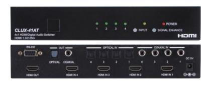
This switcher is a high performance HDMI switcher with a separate digital audio input and output. It allows you to share one HDMI display among several HDMI sources. Simply press one button to select your desired HDMI source to be displayed on the connected HDMI display, while the selected digital audio passes through Coaxial or Optical to be played on your audio amplifier.
