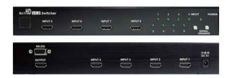
This switcher is a high performance HDMI switcher with IR remote and RS-232 controls. It allows your various HDMI sources to share one HDMI display. Simply pressing one button to select your desired HDMI source for display on the TV/monitor.
