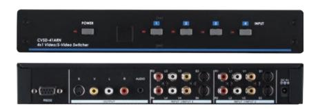
This switcher is designed to switch between various Standard-definition (SD) sources for sharing one TV/monitor. Controlled either by the input selection button on the front panel or the supplied IR remote control, this unit allows you to select your desired SD source for display on the TV/monitor with resolution up to 480i or 567i.
